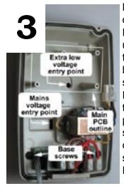
Before fitting the enclosure base ELV cabling through the opening under the circuit board and up to the top of the board. The hole can be enlarged as required with a sharp knife.
