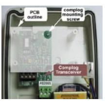
After all electrical connections have been made, with the ELV cables along the top of the main PCB and LV connections across the bottom, the enclosure cover can be fit-
