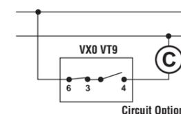
Control with "OFF" position for Heat Leakage Defrost
