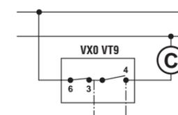
Control with "OFF" using Heater Assisted Defrost
