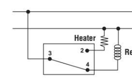
Control with Heater & Relay Controlling Compressor and By-pass Valve
