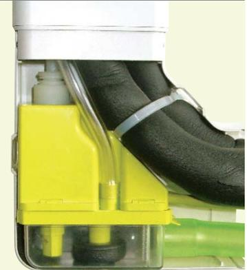
The Aspen Maxi Lime pump is completely unique, in both design and installation advantages. The pump is clipped directly onto the reservoir so there is minimal suction lift. By connecting the drain hose to the reservoir of the pump unit, condensate water can be pumped away to a suitable drain.
