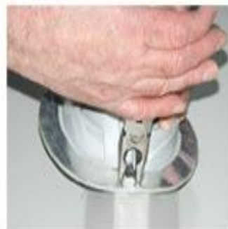
4 Crimp the clip securely closed with pliers.
