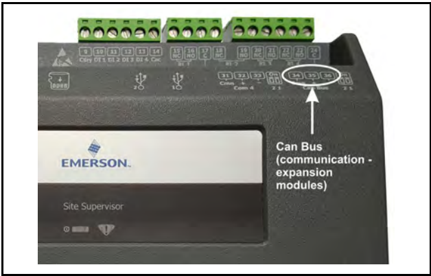
Figure 8-27 - Can Bus Expansion Module
