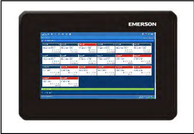
Figure 6-18 - Supervisory Controller Display
