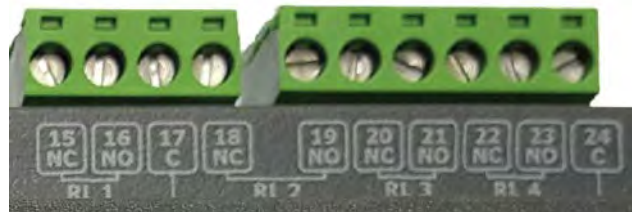
Figure 3-15 - Relay Outputs
