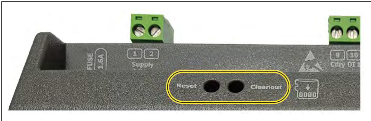
Figure H-3 - Site Supervisor Reset and Cleanout
