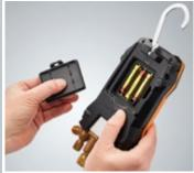
3 Loosen the 6 marked screws and remove the back of the device.
