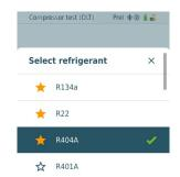
6.2 Setting the refrigerant: Press [▲] or [▼] to select the refrigerant and press [Menu/Enter] to confirm.
