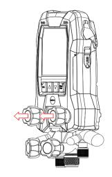
Fold out the suspension device, release the clip, remove the battery compartment cover and remove the batteries.
