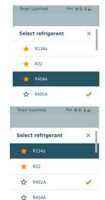
9.2 Setting the refrigerant: Press [▲] or [▼] to select the refrigerant and press [Menu/Enter] to confirm.
