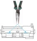
Remove the battery from the housing.
