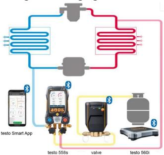
In combination with **testo 560i** and the **testo Smart Valve** the manifold **testo 558s** offers multiple functions to charge refrigerant systems.
