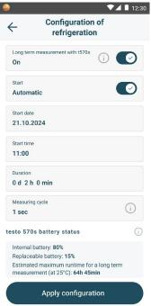
If the long-term measurement option is enabled, the configuration menu shows the remaining battery and rechargeable battery capacity and the maximum possible duration of the long-term measurement.
