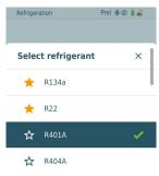
6.2 Setting the refrigerant: Press [▲] or [▼] to select the refrigerant and press [Menu/Enter] to confirm.
