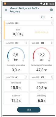
Added refrigerant is displayed in g/kg increments on the manifold/app.
