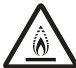
Please notice that the unit is filled with flammable gas R32. Inappropriate treatment of the unit involves the risk of severe damages of people and material. Details to this refrigerant are found in chapter "refrigerant".
