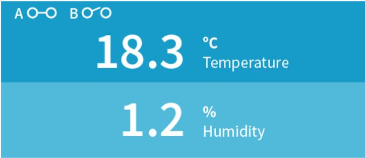
Figure 16 Relay icons on display (relay A active, relay B not active)
