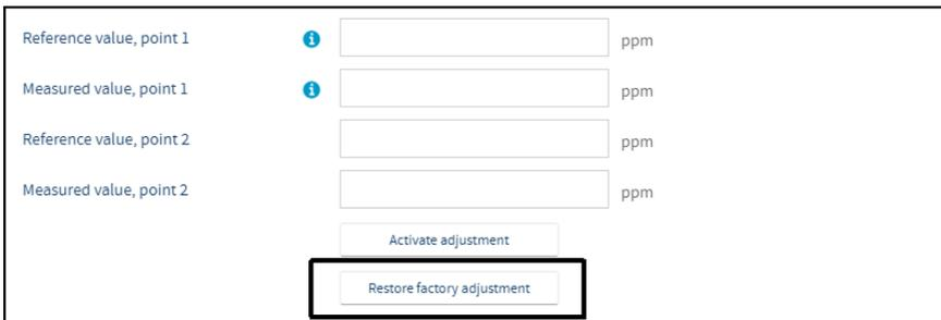
The screenshot shows the adjustment interface. It contains four rows of input fields, each with an information icon (i) to its left. The rows are labeled: "Reference value, point 1", "Measured value, point 1", "Reference value, point 2", and "Measured value, point 2". Each input field is followed by the unit "ppm". Below the input fields are two buttons: "Activate adjustment" and "Restore factory adjustment". The "Restore factory adjustment" button is highlighted with a red rectangular box.
