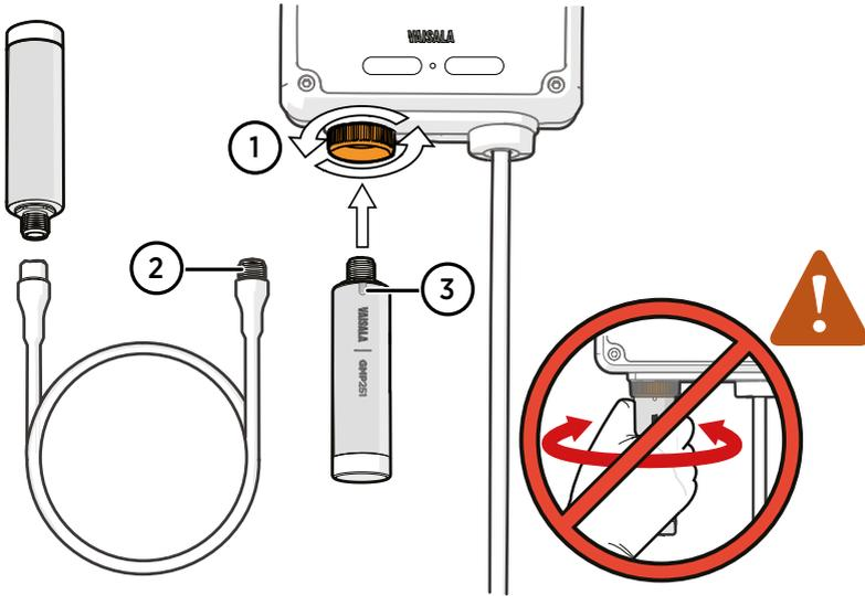
Figure 9 Attaching probes and cables to Indigo200
