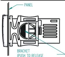
Instrument XR75CX shall be mounted on vertical panel, in a 29x71 mm hole, and fixed using the special bracket supplied. The temperature range allowed for correct operation is 0÷60 °C. Avoid places subject to strong vibrations, corrosive gases, excessive dirt or humidity. The same recommendations apply to probes. Let air circulate by the cooling holes.
