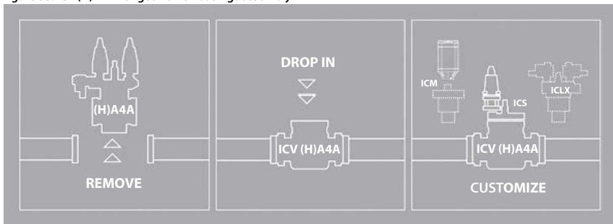
Figure 53: ICV (H)A4A flanged valve housings assembly
