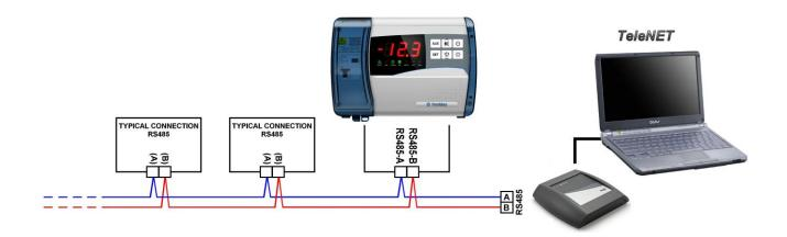
NET CONFIGURATION WITH MODBUS-RTU PROTOCOL
