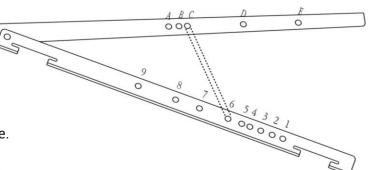
Hole C,B,A are the most commonly used hole. Hole D,E are specially made for flat roof.
