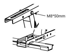
After adjusting the bracket arms' position, screw the 4 bolts of the tightening plate before placing the outdoor unit.
