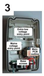
Before fitting the enclosure base over the wall mount base, feed the ELV cabling through the opening under the circuit board and up to the top of the board. The hole can be enlarged as required with a sharp knife. For maximum environmental protection, keep the hole as small as possible and later it can be silicone sealed. Similarly feed the LV mains cables through the rectangular slot, enlarging as required.
