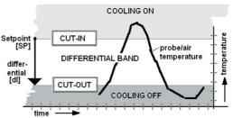
(cut out). For example: **SP** =10°C, **dI** =1.0°C: control between 9.0°C and 10°C. Another example: **SP** = 10°C, **dI** =3.0°C: control between 10°C and 13°C.
