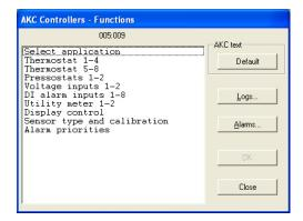
The operation is divided up into several function groups. When a selection has been made, push "OK", and you may continue to the next display. By way of example, "Thermostat 1-4" has been selected here.
