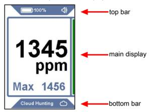
**Top bar**: The top bar includes the battery symbol, the percentage, the sensor indicator (when a non-standard sensor type is used), and the sound indicator.
