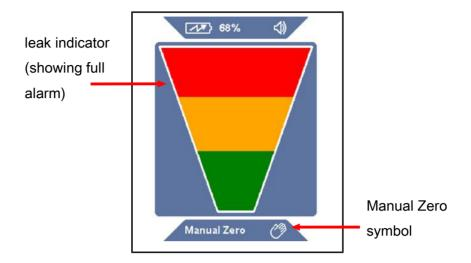
Manual Zero mode looks and operates similar to Pinpoint mode, but is identified by the text Manual Zero and the Manual Zero symbol on the bottom bar. Manual Zero mode allows the user to manually zero to the background refrigerant by pressing the SENS/ZERO button. Once the new zero point is set, D-TEK Stratus will not alarm unless a higher concentration of refrigerant is detected.
