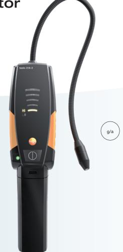
testo 316-3 is a reliable leakage detector for refrigerants which should be a part of every professional's refrigeration technology equipment. It detects even the smallest leaks thanks to its high level of sensitivity of 4 g/a, and fulfils the requirements of the F-gas regulation as well as the standards SAE J1627 and EN14624:2012.
