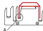
Reduce the cutting speed when the blade reaches the position A.
