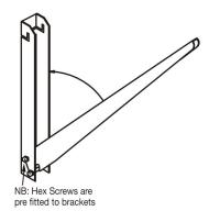
Step 2: Adjust the horizontal and vertical position of the arms, fix bracket to the wall with expansion bolts. Level vial is needed to align the 2 arms.
