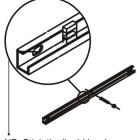
NB: Stick the liquid level here when installing (optional)
