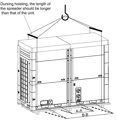
During transport by the forklift ,the symmetric holes should be used at the A-A or B-B base of the unit itself, or at the wooden base.
