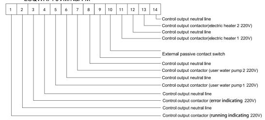
Note: the output control lines of the AC contactors for the running indicator, water pump 1, water pump 2, auxiliary electric heater 1, auxiliary electric heater 2 can be wired to the
