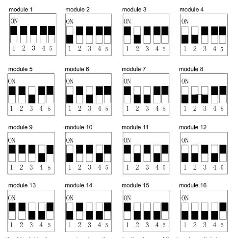
Note: the black block represents where the projecting lever of the toggle switch is.
