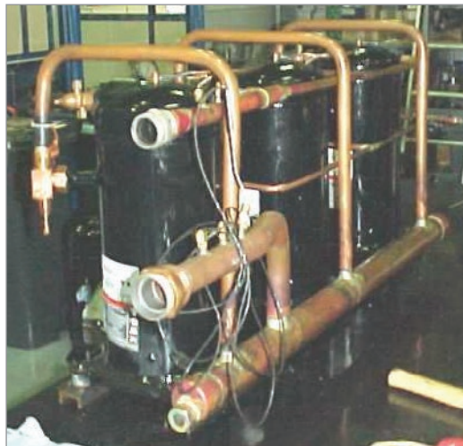
Figure 3: Suction line configuration
