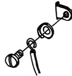
Figure 2 O18 Electrical Terminals
