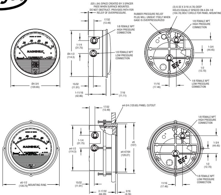
\*The blowout plug is not used on models above 180 inches of water pressure, medium or high pressure models, or on gages which require an elastomer other than silicone for the diaphragm.
