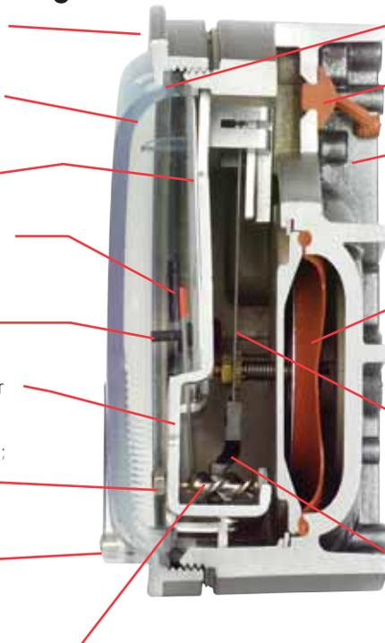
**O-ring seal** for cover assures pressure integrity of case.
