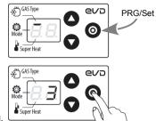
PRESS PRG/Set for 2 seconds to accept and enable the control.
