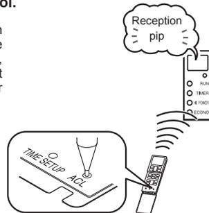
**3** Check that the reception buzzer sound "pip" is emitted from the indoor unit.
