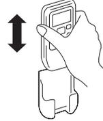
For installing or removing the remote control, move it up or down in the holder.
