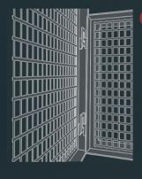
Stand RIGHT SIDE PANEL of the guard on its edge with wall mount plate facing up
