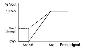
If the input signal is higher than the Set, the output signal is 230 Volt (fans are running at the maximum speed). When the signal decreases and enters the range between the Set and Set-Diff the output signal follows the temperature variation. Below the Set-diff value the output signal is always 0V (if no Vmin has been set).
