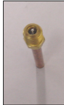
Schraeder valve with core in place
