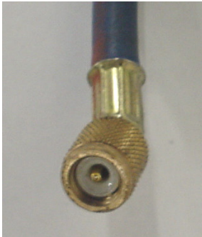
Hose with Schraeder valve Depressor
