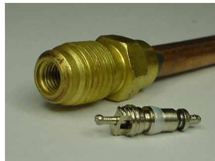
Schraeder valve with core removed
