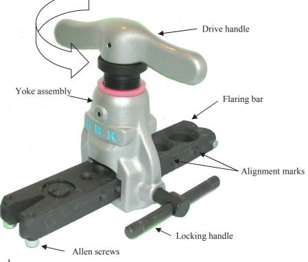
When not in use it is advisable to have a short length of flared copper tube placed in one of the flaring cutouts. (we supply the bar this way) Align the yoke with the cutout using the alignment marks as discussed and <u>gently</u> position the cone onto the copper by rotating the handle. Do not tighten the flare, the aim here is to provide support to the yoke in case the unit is accidentally dropped.
