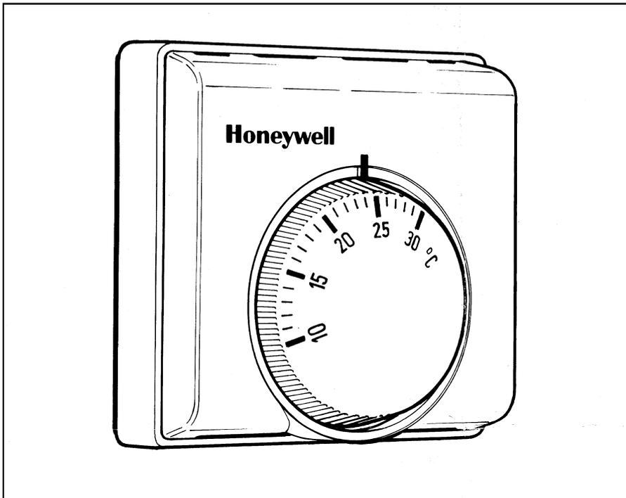
The T4360/T6360 range of thermostats are designed to provide automatic ON/OFF control for gas valves, circulation pumps, relays and zone valves in all heating, cooling, or heating/cooling installations where single or changeover switching up to 10 A (resistive load) or 3 A (inductive load) is required.
