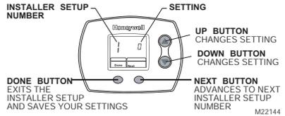
Fig. 18. Review thermostat buttons used for Installer Setup.
