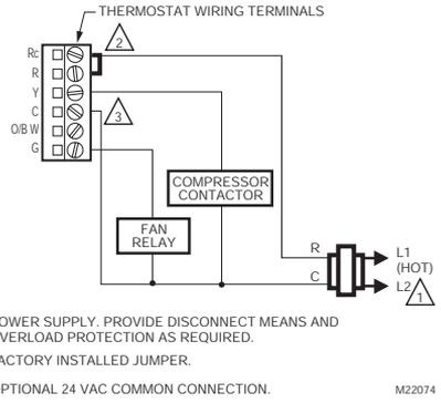
Fig. 12. Typical hookup of cool only system.
