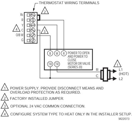
Fig. 11. Typical hookup of heat only Series 20 system.
