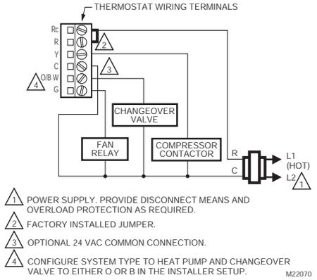
**Fig. 8. Typical hookup of 1H/1C heat pump.**
