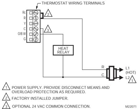
**Fig. 9. Typical hookup of heat only system.**
