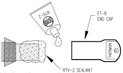
3 Slide the end cap onto the cable with a twisting motion, making sure to work out any air pockets. Wipe off the excess sealant. Pull the braid over the end cap & then crimp together the braid ends with the 8-AWG compression lug supplied.
